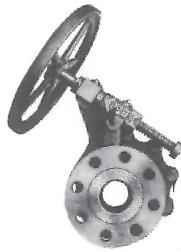
Line pressure and heavy spring hold disc firmly against the body seat, sealing off the flow. When operated, the disc slides across the body seat pushing harmful boiler scale away, and wiping clean the precision lapped surfaces.
