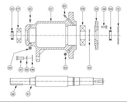
NOTE: Note difference in visual appearance of bearing frames on pages 2 and 3. New frames are a direct replacement for older ones. The part numbers for individual bearings are different from old frames to new frames. If you need help determining which frame you have, please contact tech services at Taco (401-942-8000).
