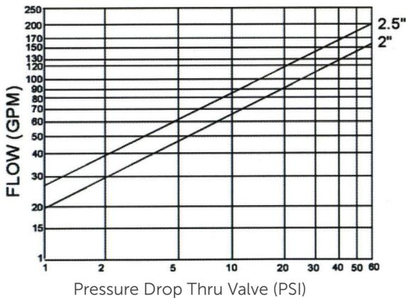
All flow capacities are based upon a 24 degree F max temperature rise above valve opening point.
