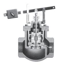
The No. 73 Single Seated Lever Valve is the same as No. 7, shown and described on pages 7 and 8, minus float, float rod and rosette, and plus a counterweight.
