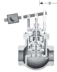
The No. 773 Single Seated Lever Valve is the same as No. 77, shown and described on pages 7 and 8, minus float, float rod and rosette, and plus a counterweight.
