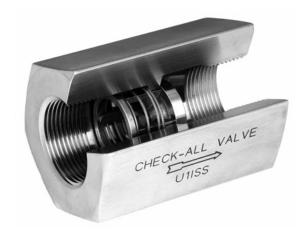
The Universal High Pressure (U1) check valve is a one piece body machined from bar stock with female pipe threads. The valve is designed and manufactured for high pressure applications. This valve is normally supplied with a metal "to" metal seat. Also available with ISO 7 "Rp" threads. (R1)
