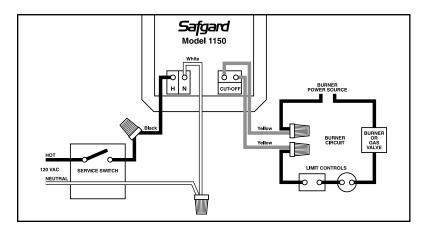
Connect the black wire **(H)** from the Safgard 1150 to the hot 120 VAC lead coming from the service switch. Connect the white wire **(N)** to the neutral 120 VAC lead. Locate and break into the burner circuit. Connect the yellow wires **(CUT-OFF)** from the Safgard 1150 in series with other limit controls as shown.
