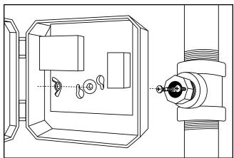
Remove wing nut from the probe terminal. Mount the control box on the probe by aligning the keyhole slots with the mounting screws. Replace the wing nut. Secure the control box by tightening wing nut and two mounting screws.
