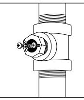
Apply pipe sealing compound to probe threads and install in boiler or tee. Tighten so that the mounting screws are horizontally aligned.
