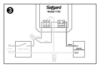
**Step ③** Connect the second yellow wire (CUT-OFF) from the Safgard 1150 to the (L1) boiler connection.
