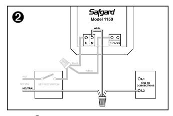
**Step 2** Connect the white wire (N) from the Safgard 1150 to the neutral 120 VAC lead and to the (L2) boiler connection.
