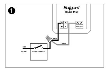
**Step 1** Connect the black wire (H) and one of the yellow wires (CUT-OFF) from the Safgard 1150 to the hot 120 VAC lead coming from the service switch.
