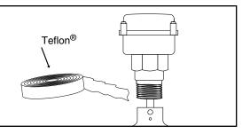
**c.** Insert the flow switch into the pipe tee. Turn the flow switch two (2) or three (3) revolutions clockwise until tight. Do not put excessive force on cover when turning.
