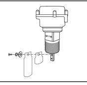
**b.** Apply pipe sealing compound or Teflon® tape to the flow switch pipe threads.
