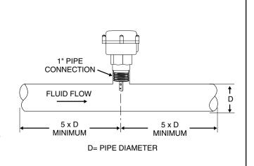
a. The flow switch must be installed in the pipe using a threaded tee connection or welding fitting of minimum length such as a half coupling. Use a face or hex bushing to reduce the tee outlet to 1" pipe thread if a reduced tee outlet thread size fitting is not available.
