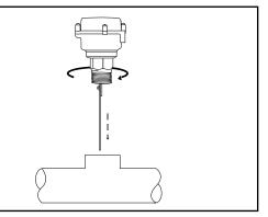
d. Place a 1 3/8" open end wrench on flow switch body to tighten to final position. Final position is with arrow on body aligned in the same direction as liquid flow.
