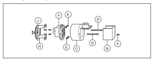
Conduit housing is movable into any one of four positions. Remove two screws (D) and rotate to desired position. NOTE: 11M cannot be rotated out of "TOP" position due to reset button orientation requirement.
