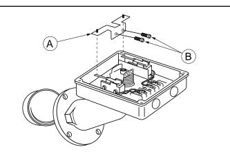
**6.** Remove the two Torx® screws (C) holding the switch bracket assembly in place using a flat head screwdriver or a Torx® T30 wrench.
