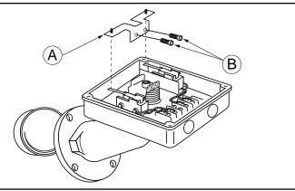
10. Reconnect the pump switch and burner/ alarm switch wires to terminal block as noted when disconnected and torque to 13 - 17 in. lb. (15 - 19.5 cm. kg.) (Refer to "Terminal Connection Chart" on page 5 if unsure of proper switch to terminal block wire connections).
