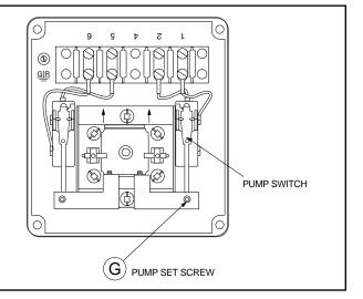
**5d.** Slowly drain the water in the boiler until the pump turns on. Allow pump to fill the boiler and observe the point on the ruler where the water level shuts off.
