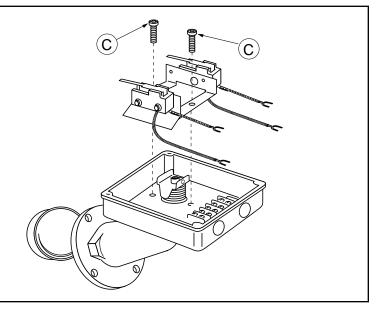
7. Take the new switch bracket assembly out of the package and place the bagged supplies to one side while discarding the insert.
