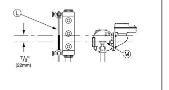
c. Continue watching the gauge glass (L) to see that the water continues to rise to approximately 1%" (35mm) above the horizontal cast line (M). The pump should shut off.
