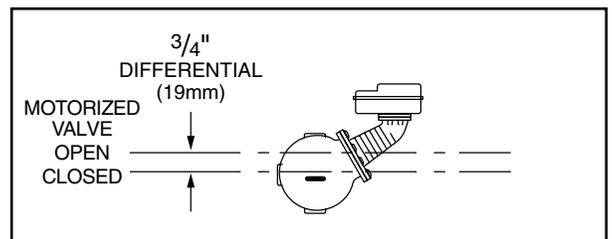
NOTE: Due to the slower operation of some motorized valves, complete valve opening or closing will occur at slightly different levels than indicated above.
