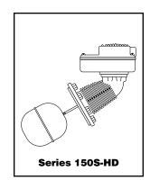
Head mechanisms include a gasket and bolts. (S) in model number indicates snap switch.
