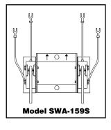
Switch assemblies include a mounting bracket and color-coded terminal connection wires.
