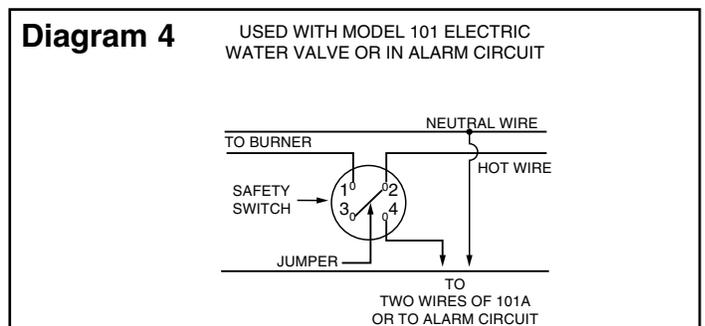
**IMPORTANT:** Low water cut-off circuit of the 69 series must be electrically wired in series with all other boiler limit operating controls.
