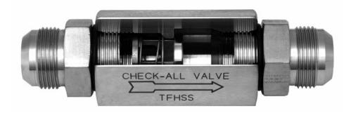
The Tubing Check Valve-Flared (TF) is a three-piece constructed check valve with 37° flared end fittings that conform to SAE J514 & ISO 8434-2. These valves are designed for maximum flow with minimal pressure drop. Consult the factory for more information.
