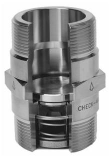
The **Connector (CN)** valve is a check valve with a hex nipple or connector housing. It is designed to be used in installations where a check valve with male pipe threads are required. The Connector valve is adaptable for use as a check valve, vacuum breaker, or low pressure relief valve. Two valves used in combination make an excellent low pressure relief/vacuum breaker. Also available with ISO 7 "R" threads.
