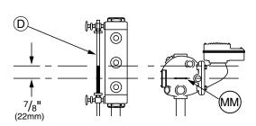
c. Continue watching the gauge glass (D) to see that the water continues to rise to approximately 13%" (35mm) above the horizontal cast line (MM). The pump should shut off.
