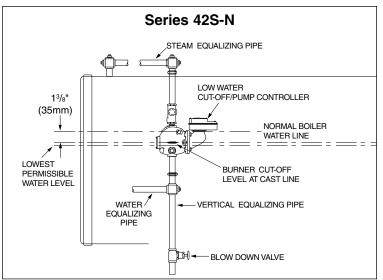
The 42S-A controls are installed in boiler's gauge glass tappings. The horizontal cast line should be approximately 1" (25 mm) above the bottom of the glass. Verify that this level is not below the lowest, safe permissible water level, as determined by the boiler manufacturer.
