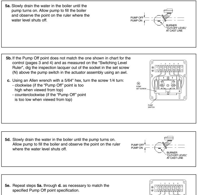
f. Apply one drop of adhesive (furnished) to the set screw threads (O) above the pump switch in the actuator assembly.
