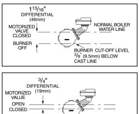
NOTE: Due to the slower operation of some motorized valves, complete valve opening or closing will occur at slightly different levels than indicated above.
